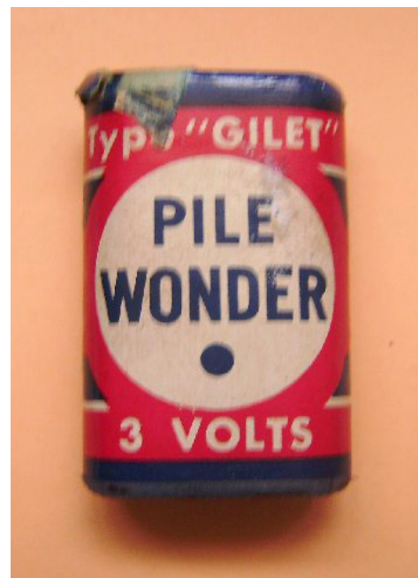
Old 3 V zinc-carbon battery (around 1960), with cardboard casing
